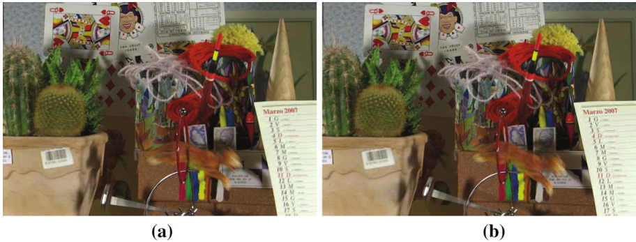
Fig. 6 The reconstructed video frames—“Cactus” (23rd frame, QP=22) under low delay setting a original HEVC (SSIM: 0.9956, GMSM: 0.9005, GMSD: 0.1694, bits: 260,504 bits); b proposed method (SSIM: 0.9952, GMSM: 0.9056, GMSD: 0.1762, bits: 221,536 bits)
